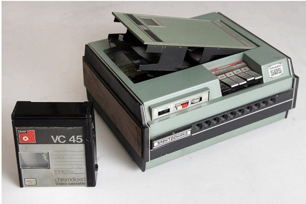
Soviet video cassette recorder “Elektronika-505 video” with BASF cassette of “VCR” format in Nizhegorodskaya radio laboratory Museum exhibition.
